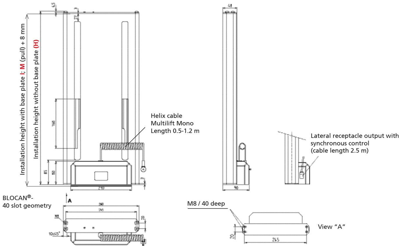
Base plate **(I)** with fixing plates (4 counterbores)
