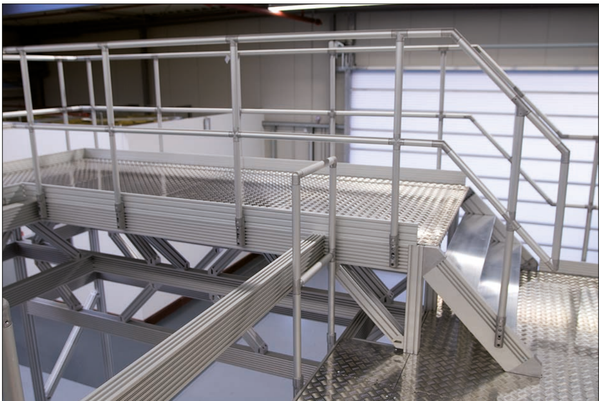
Maintenance platform at printing machine ( internal tension system )
