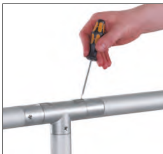
Release stopper with a screwdriver
