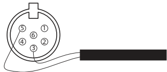
DIN 45322 plug – Connection of PIN3 and PIN5 to the switch strip
