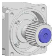
4. Fit the washer into the toothed washer.
